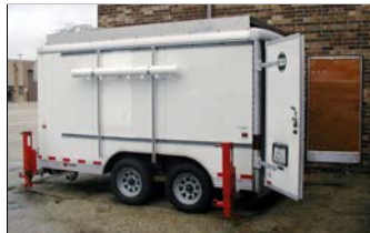
Mobile groundwater remediation system - turnkey package installed in 48' trailer for air / ozone sparging 60 injection wells at a Superfund site. Cleanup was achieved and system moved to another site.
