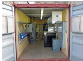
Stationary groundwater remediation system with 24 lbs/day ozone - turnkey package installed in 20' cargo container for air/ozone sparging at 80 injection wells, with PLC for user adjustable timing of pulsed sparging.
