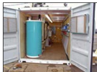
Stationary groundwater remediation system with 24 lbs/day ozone - turnkey package installed in 20' cargo container for air/ozone sparging at 80 injection wells, with PLC for user adjustable timing of pulsed sparging.
