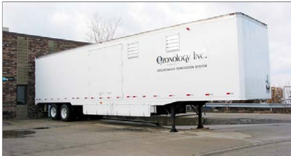
Mobile groundwater remediation system - turnkey package installed in 48' trailer for air / ozone sparging 60 injection wells at a Superfund site. Cleanup was achieved and system moved to another site.
